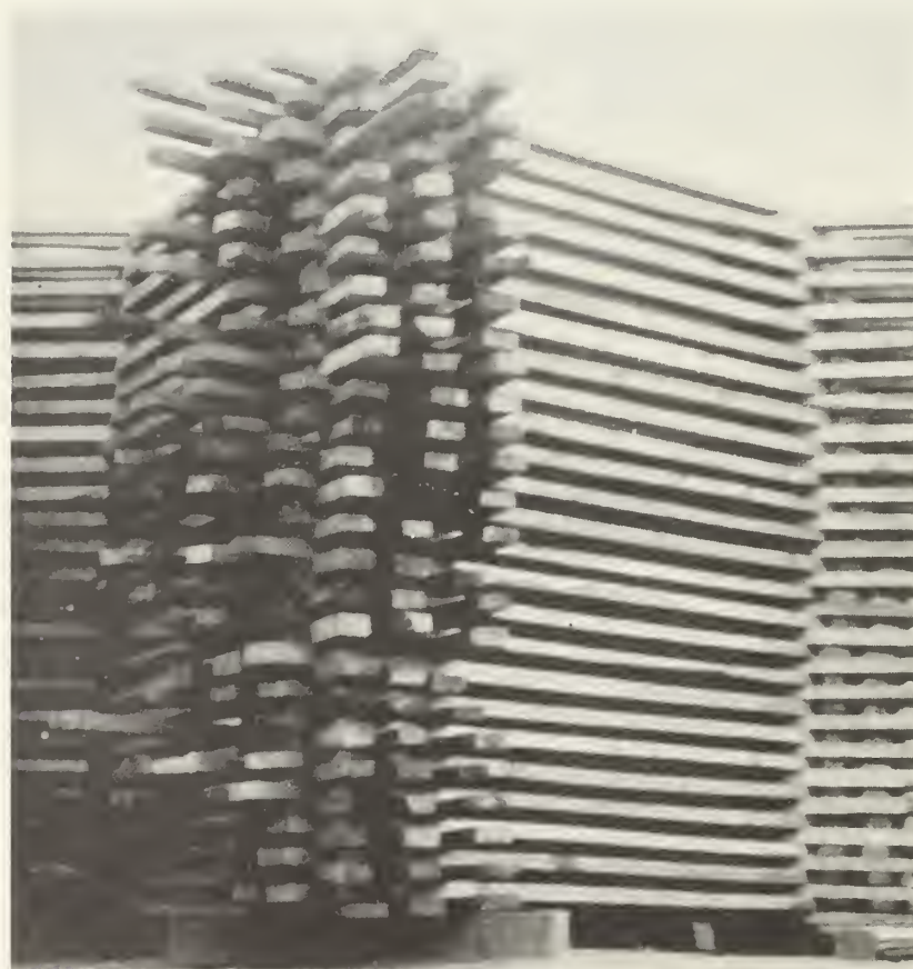
Figure 22. --Crib piling of 2 by 4's.
